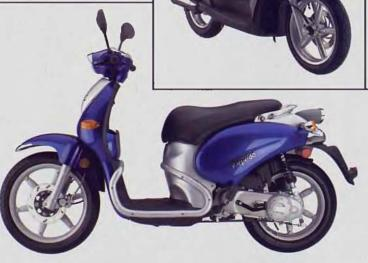
Above: The Torpedo 125cc 4t scooter by Italjet includes passenger footpegs and a rear grab rail for the rider in back. Stash your helmet in the storage space under the seat. (Price: about \$3800.) Right: Piaggio originally sold the LT 150cc in Europe under the name Liberty but recently introduced it to the U.S. The four-stroke engine is fuel-efficient and extremely quiet. Chrome-plated sidebars and springs, a large seat and an electronic antitheft immobilizer are standard (\$3400).
